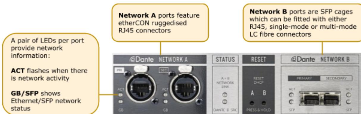
The SB 32.24 and SB 16.12 have two sets of redundant network connections. These can be configured in two different modes:
