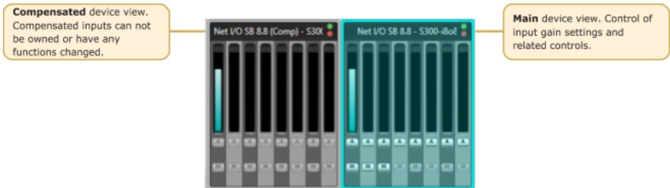
The compensated output's level is controlled in the stagebox itself, so any Dante device can receive the compensated signal, it does not have to be an SSL console.
