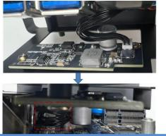
Store the wires within the space between the large capacitor
