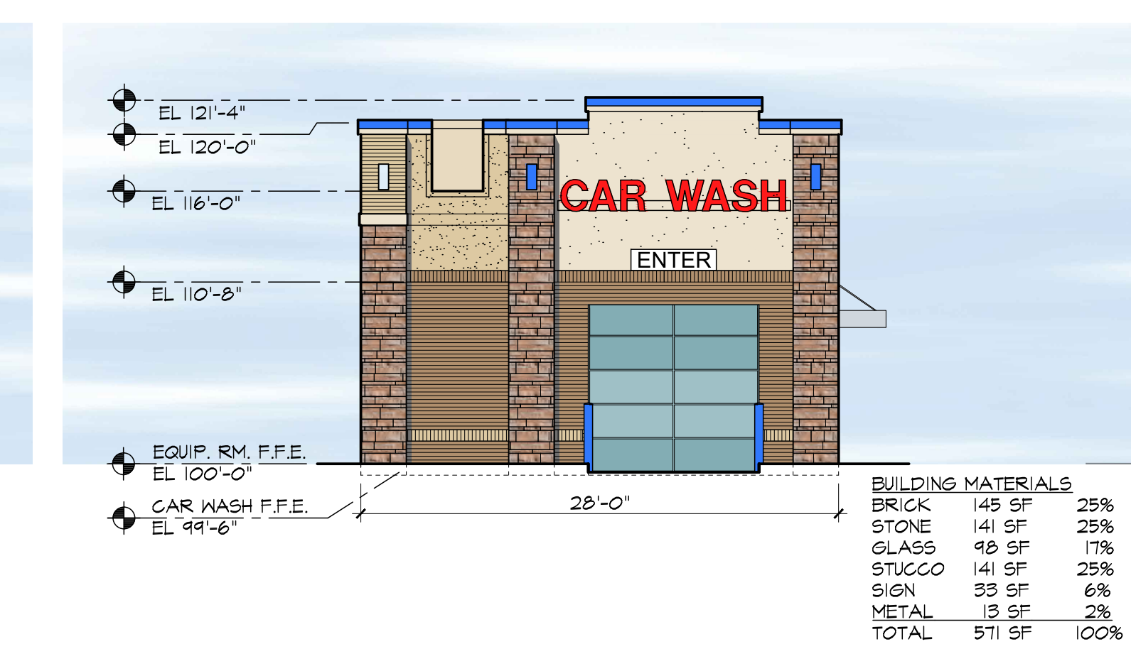
4 EAST CAR WASH ELEVATION 1/8" = 1'-0"
