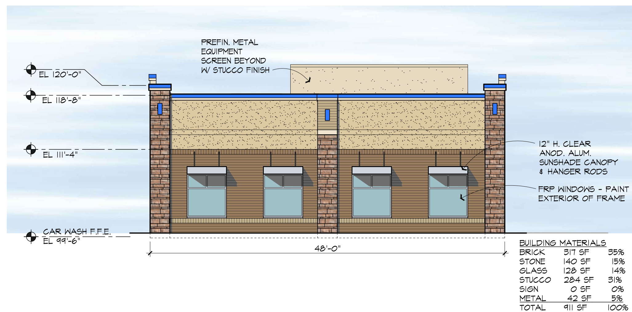
1 NORTH CAR WASH ELEVATION 1/8" = 1'-0"
