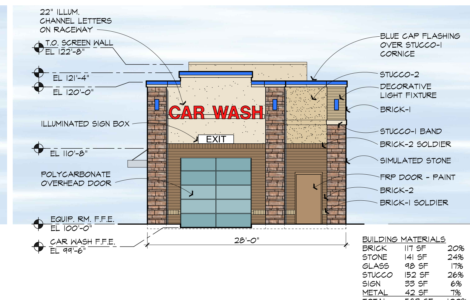
2 WEST CAR WASH ELEVATION 1/8" = 1'-0"
