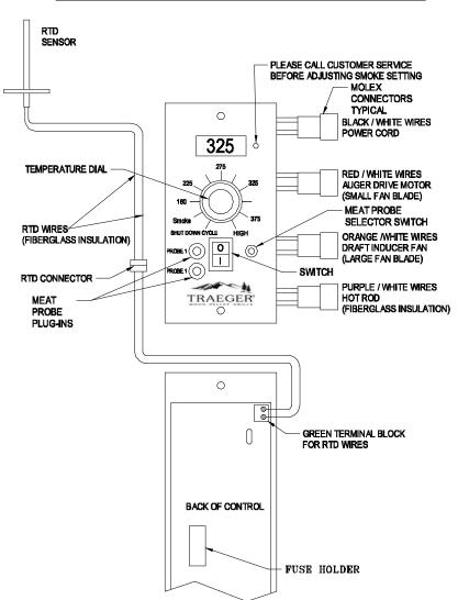
DIGITAL THERMOSTAT CONTROL WIRING DIAGRAM
