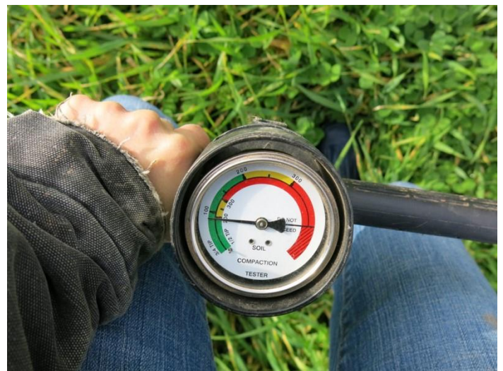
Figure 6. When the dial on a penetrometer reaches 300 psi compaction levels are restricting root growth. Photo credit T. DuPont, WSU Extension.
