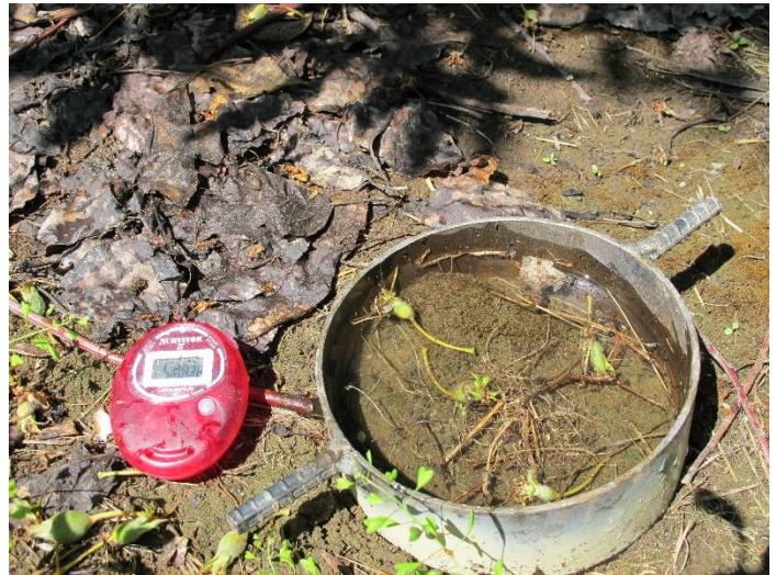
Figure 7. Water infiltration can be measured with a simple metal ring and a stop watch. Photo credit T. DuPont, WSU Extension.
