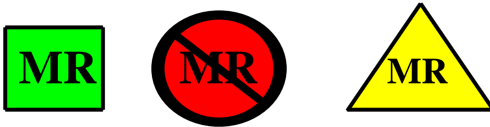
Fig. 2: U.S. Food and Drug Administration labels (developed by ASTM [American Society for Testing and Materials] International) for portable objects taken into Zone IV. The square green “MR safe” label is used for wholly nonmetallic objects, the triangular yellow label is used for objects with “MR conditional” rating, and the round red label is used for “not MR safe” objects.
