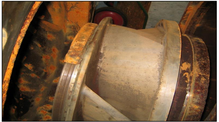
Example of bacterial corrosion on a suction wear ring of an impeller
