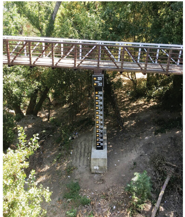
Visible stream gauges were placed at various locations along Coyote Creek to provide "real-time" information on water levels.
