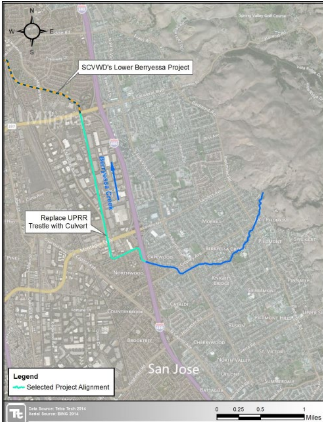
Figure 6 – Selected Project Alignment, Earthen Trapezoidal Channel, Completed 2019
