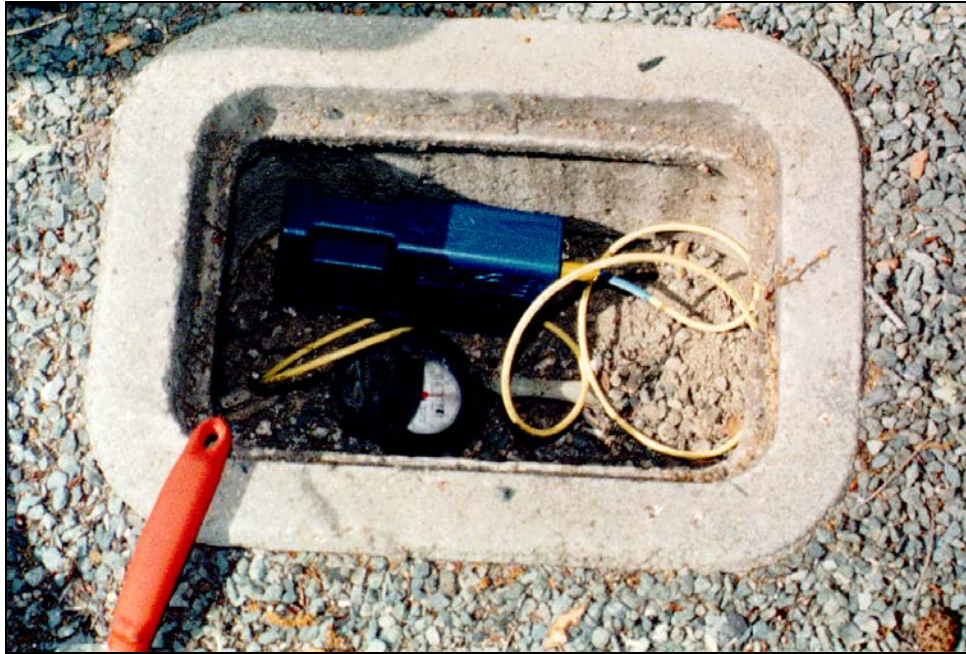
Figure 2: Example of a data logger installed on a residential meter (photo supplied by Aquacraft, Inc.)
