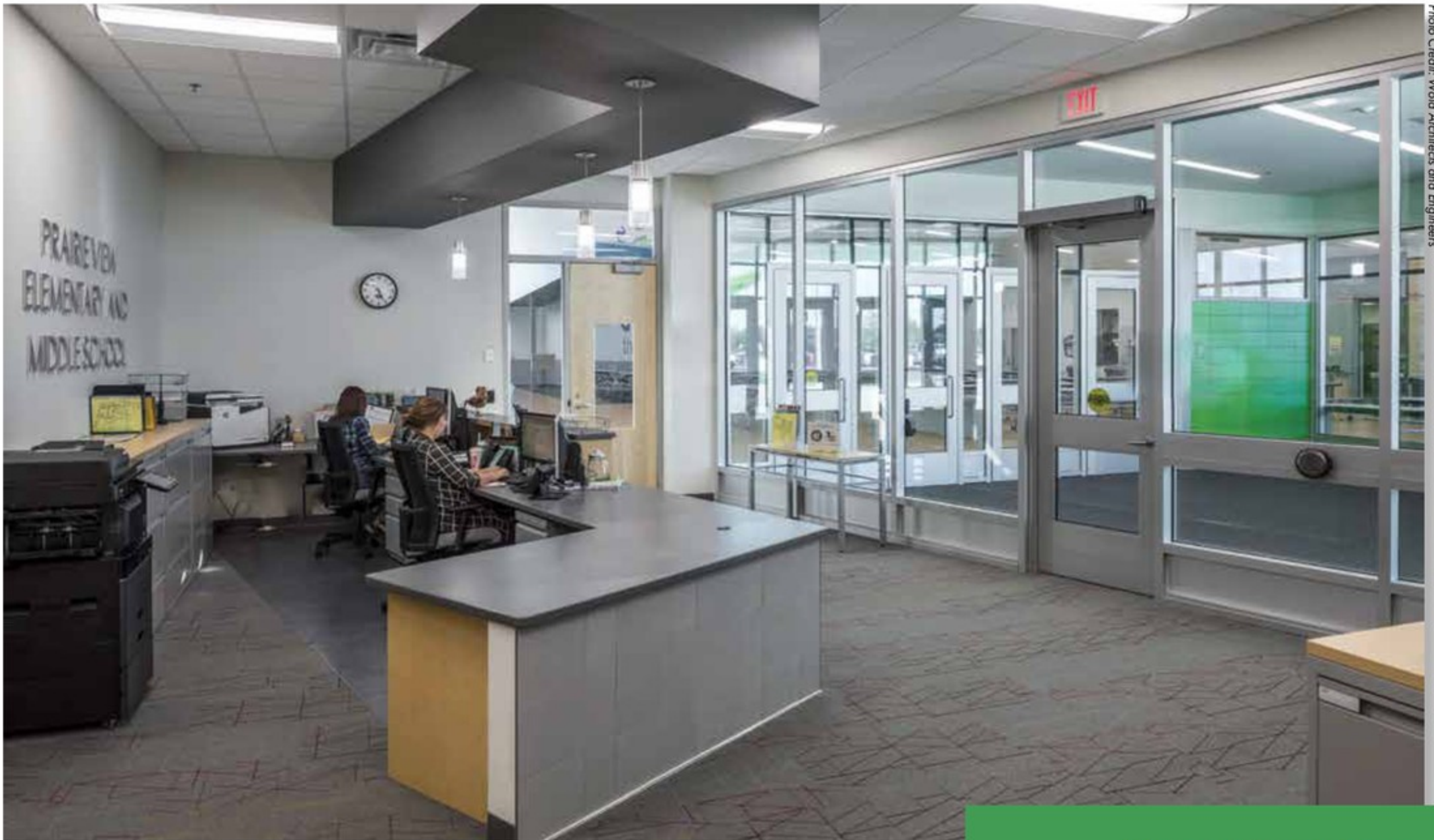
Prairie View Elementary and Middle School (Minn.) secure vestibule, designed by Wold Architects and Engineers; the space's visibility, double doors, electronic locks/intercom, and hardened materials allows staff to safely screen visitors before they enter.
