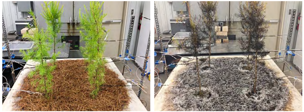
Figure 2. Laboratory burn experiment to evaluate post-fire physiological performance of western larch ( Larix occidentalis ) seedlings. Photos show seedlings before (left) and after (right) a high fire radiative energy density (FRED) burn treatment ( 1.2 \text{ MJ m}^{-2} ). More details on these seedlings and experiments are found in Smith et al. (2017). Photos: Alistair Smith.
