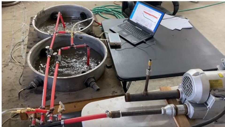
Figure 1. (top) Schematic of experimental set-up for weathering of basalt to be used in Tasks 2 and 3; (bottom) The weathering system in operation (schematic and photograph by David Drinkard)
