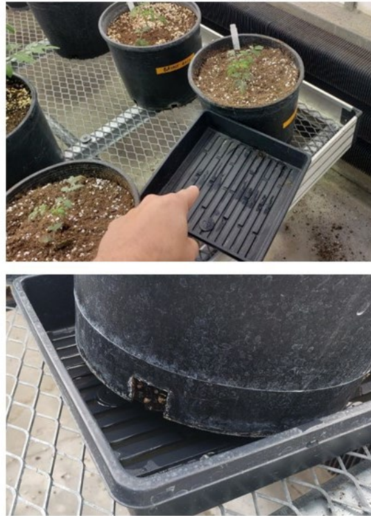
Figure 5. (top) Plastic trays used to collect pot leachate samples; (bottom) close-up view of leachate tray under pot
