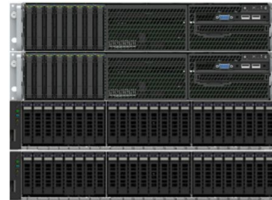
2x Intel S2600WFT Servers
